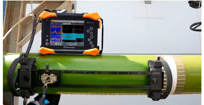
Figure 5: LYNCS scanner for weld inspection and corrosion mapping.
