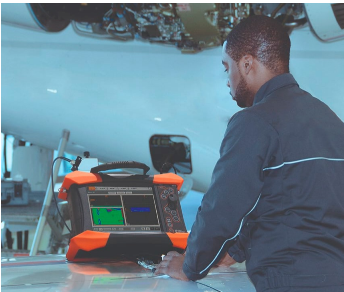
Figure 1: Gekko performs aerospace composite material inspection.
